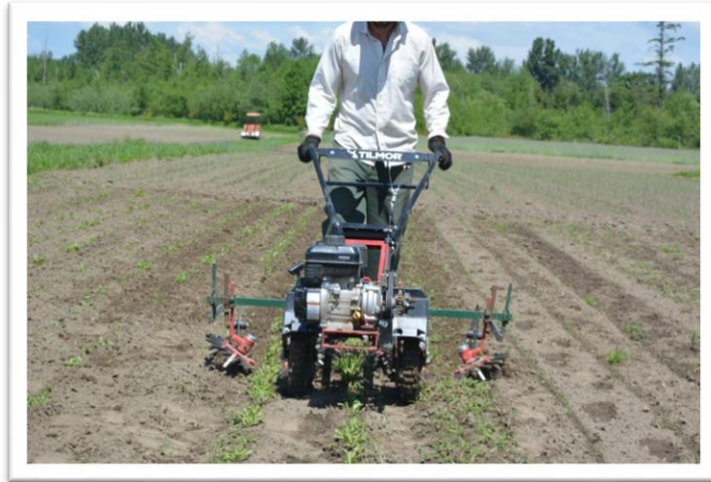
Walk behind Skeetee 2-row finger weeder. Weeding tools are mostly the same for beet and carrot production.
