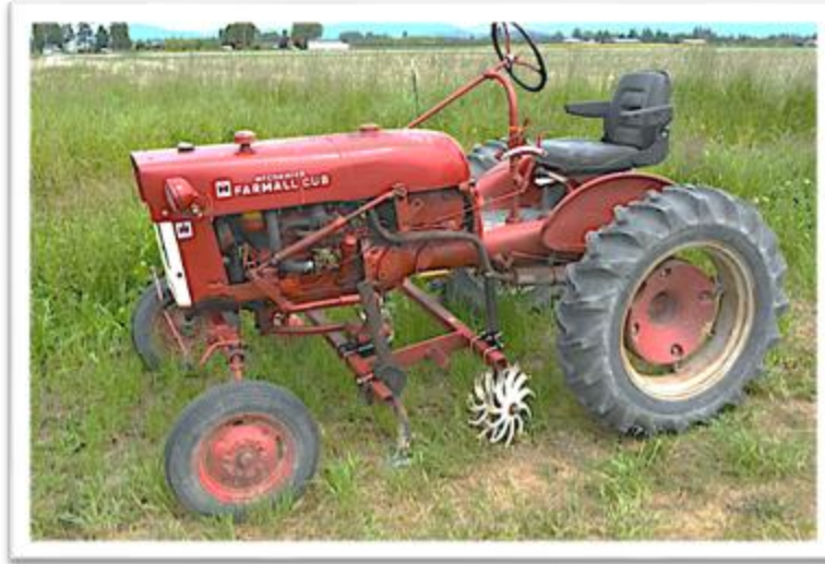
Farmall setup for alleyway/ poly film edge cultivation
