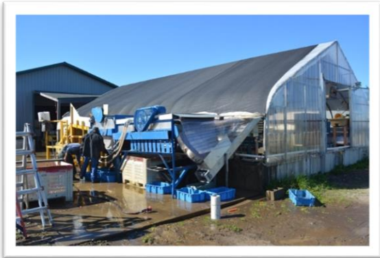
L: Outside bin dump and wash process for carrot and beet line
