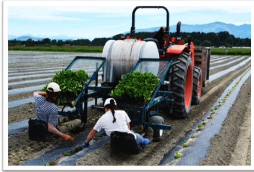
Poly-mulched beds: Water Wheel transplanter punches whole in poly depositing water and fertilizer at the same time.
