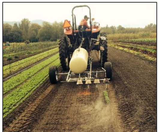
High-density Seeder rolls out flat seed bed
