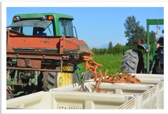
L: Macro bins hold about 700 lbs. of Carrots R: Bin loader has conveyor can pick up 4 bins and unload 4 bins from tractor
