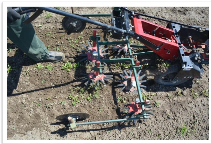
Versital walk behind cultivation tool. Hybrid Tilmor brand walk behind using Skeetee cultivating heads.
